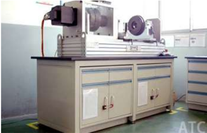
Torque-tension-friction tester from Germany
