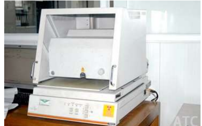
German X-Ray coating/plating film tester
