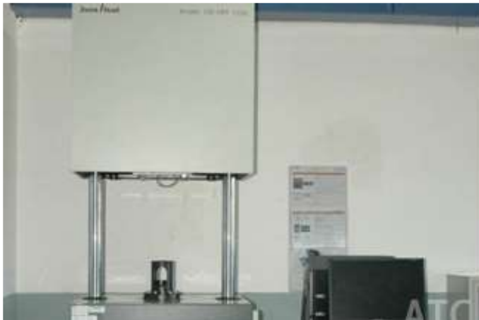
Swiss made high frequency fatigue tester
